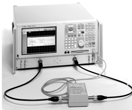
Calibration configuration using the PNA series
